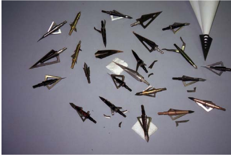
Some of the broadheads damaged during 2004 testing.
