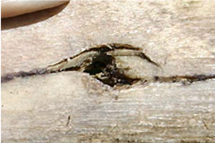
Single bevel induced rotation is clearly visible.
